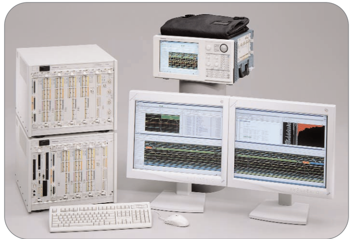
► Figure 3: TLA715 with internal display and TLA721/7XM with optional dual 21" flat-panel monitors.
